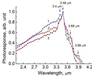
Fig. 4. Photoreponse spectrum of the QD PCC at different biases: 1 – 6 mV, 2 – 2 mV, 3 – 1 mV.
