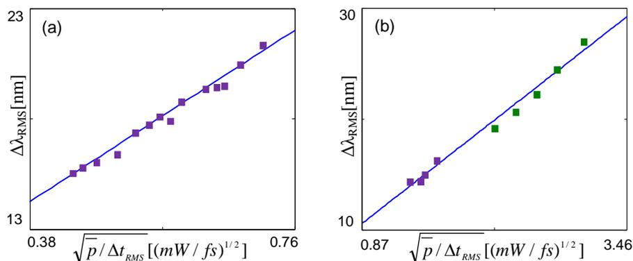
Fig. 3. (a) experimental results on the similaritonic technique for pulse duration measurements for compressed pulses, and (b) comparison of the similaritonic technique for compressed pulses and laser pulses.
