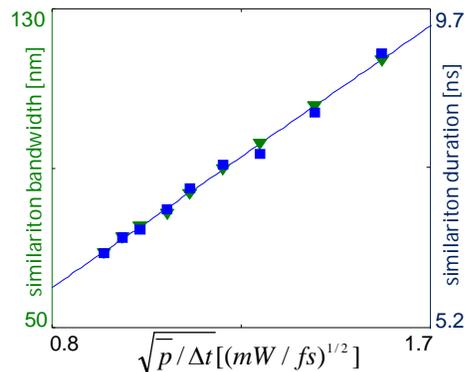
Fig. 2. Experimental results on the similaritonic technique for pulse duration measurements for stretched laser pulses. The green triangles and blue squares correspond to spectral and temporal measurements of the similariton, respectively.
