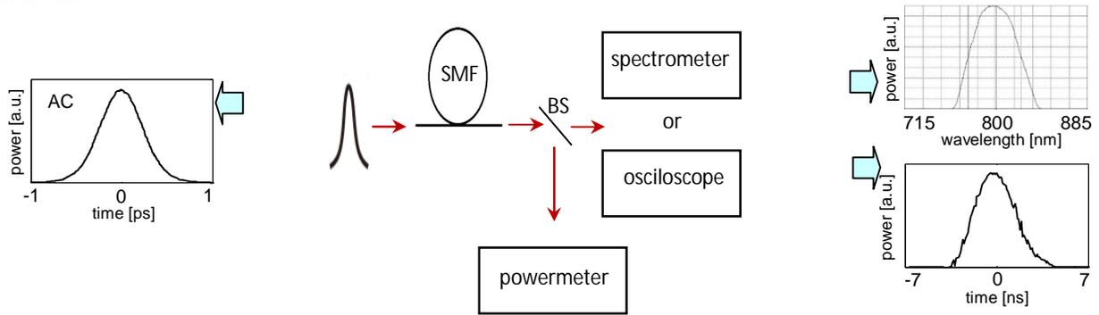
Fig. 1. Experimental setup of the similaritonic technique of duration measurements.
