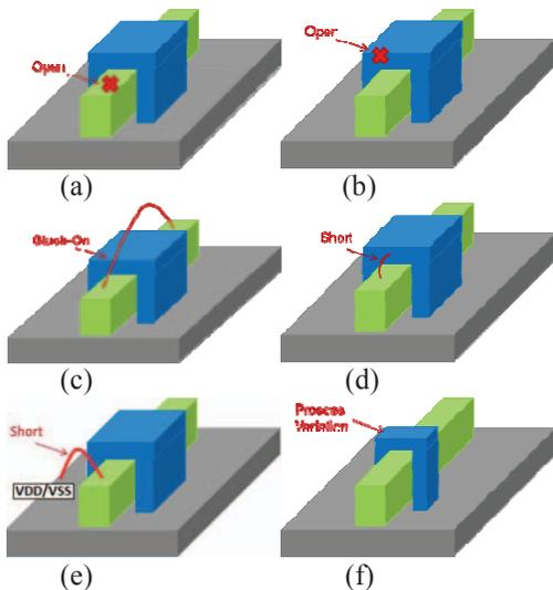
Figure 3. Defect models considered for FinFETs
