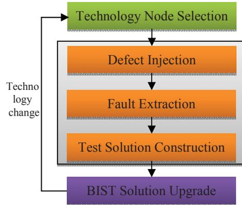
**Figure 2. Test methodology development flow for embedded memories**
