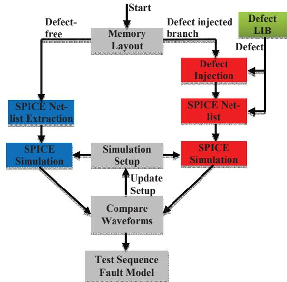
Figure 4. Defect Injection and Fault Modeling Flow
