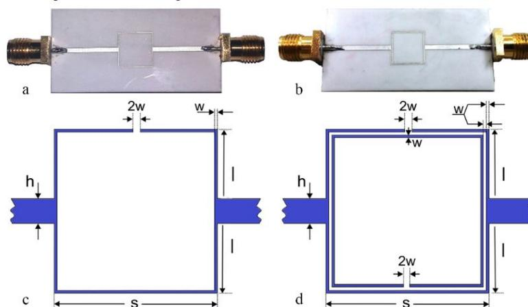
Fig. 1. The real images of prepared (a) single rectangular and (b) double rectangular resonators. The structural geometry of (c) single rectangular and (d) double rectangular resonators.
