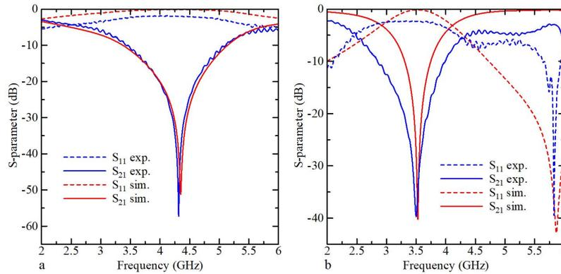
Fig. 3. The obtained experimental and simulation S-parameters without MUT for (a) single rectangular resonator and (b) double rectangular resonator.
