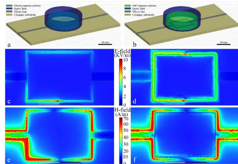
Fig. 2. The computer models in HFSS for (a) single rectangular and (b) double rectangular resonators. Simulated electric field distribution for (c) single rectangular and (d) double rectangular resonators and simulated magnetic field distribution for (e) single rectangular and (f) double rectangular resonators without MUT.
