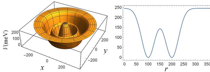
Fig. 1. The 3D (left) and 2D (right) plots of the confining potential of DQR. The Cartesian coordinates “ $x$ ” and “ $y$ ” and the radial coordinate “ $r$ ” are expressed in angstroms.
