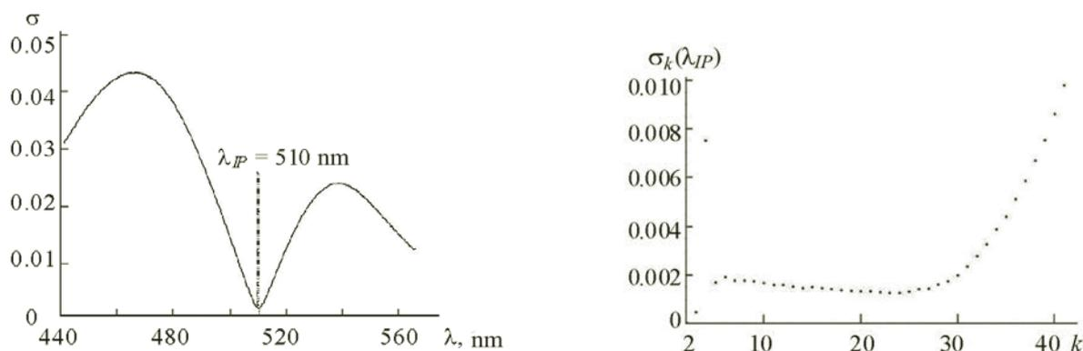
Fig. 2. Mean-square deviation of the absorption vs. wavelength  $\sigma(\lambda)$ , calculated using formula (3), for all the spectra ( $k = N = 40$ ).
