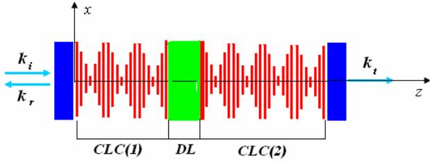
Fig. 1. A sketch diagram of a modelled CLC cell with a defect layer inside.
