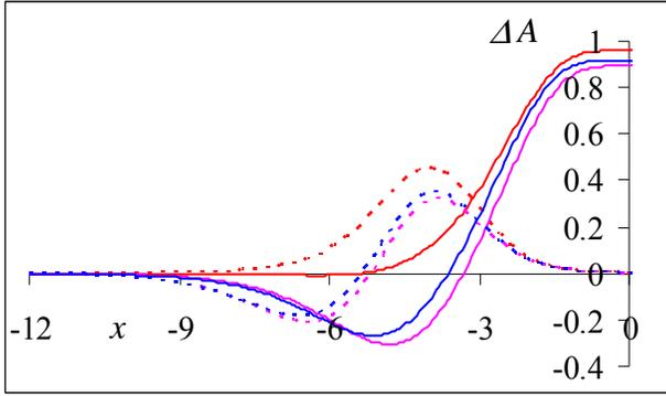
Fig 3. The circular dichroism ( $\Delta A$ ) versus the parameter,  $x = \ln(\text{Im} \epsilon_m)$ , characterizing the absorption at different values of the defect layer thickness.
