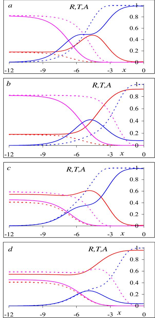
Fig. 4. The dependences of the reflection (the red lines), transmission (the pink lines) and absorption (the blue lines) on  $x = \ln(\text{Im} \epsilon_m)$ . The solid lines correspond to the right circular polarization of the incident light and those dashed to the left circular polarization. *a, c*:  $n_o''=n_e'' \neq 0$  and  $n''=0$ ; *b, d*:  $n_o''=n_e''=0$  and  $n'' \neq 0$ . *a, b*:  $d_2=2100$  nm,  $\lambda=617.5$  nm, *c, d*:  $d_2=2000$  nm,  $\lambda=625.5$  nm.
