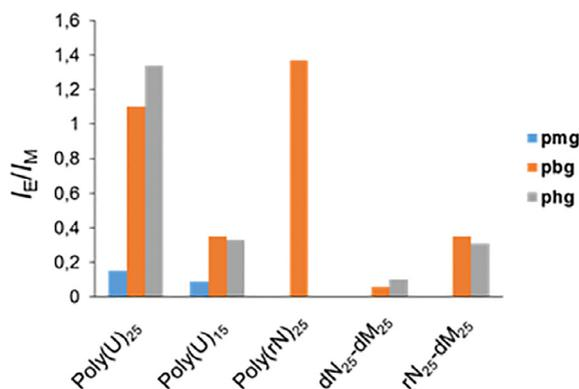
**Fig. 6.**  $I_E/I_M$  maximum values obtained for **pmg**, **pbg** and **phg** (50  $\mu$ M) mixed with various RNA sequences and duplexes. Experiments were performed in MOPS buffer (1 mM MOPS and 1 mM NaCl) at pH = 7.5.
