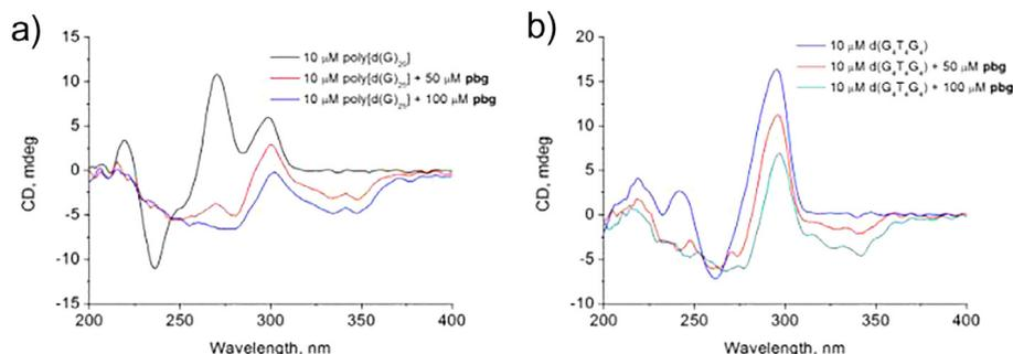
**Fig. 5.** CD spectra of a) parallel quadruplex structure poly(dG)<sub>25</sub> (10  $\mu$ M) and b) anti-parallel quadruplex structure G<sub>4</sub>T<sub>4</sub>G<sub>4</sub> upon the addition of **pbg**. Experiments were performed in MOPS buffer (1 mM MOPS and 1 mM NaCl) at pH = 7.5.
