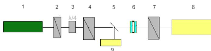
Fig. 2. The experiment diagram. (1) Diode-pumped solid-state LASER, (2)  $\lambda/4$  slab, (3) circular pole, (4) linear pole, (5) mirror, (6) cell, (7) analyzer, (8), (9) recorders.
