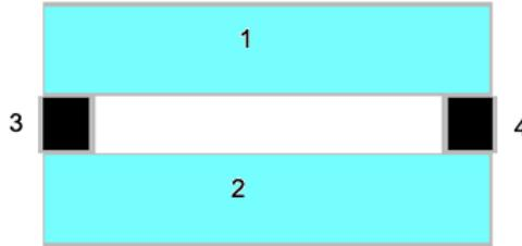
Fig. 3. Cell appearance of 1.2 glass stands 3 and 4 plastic spacers.
